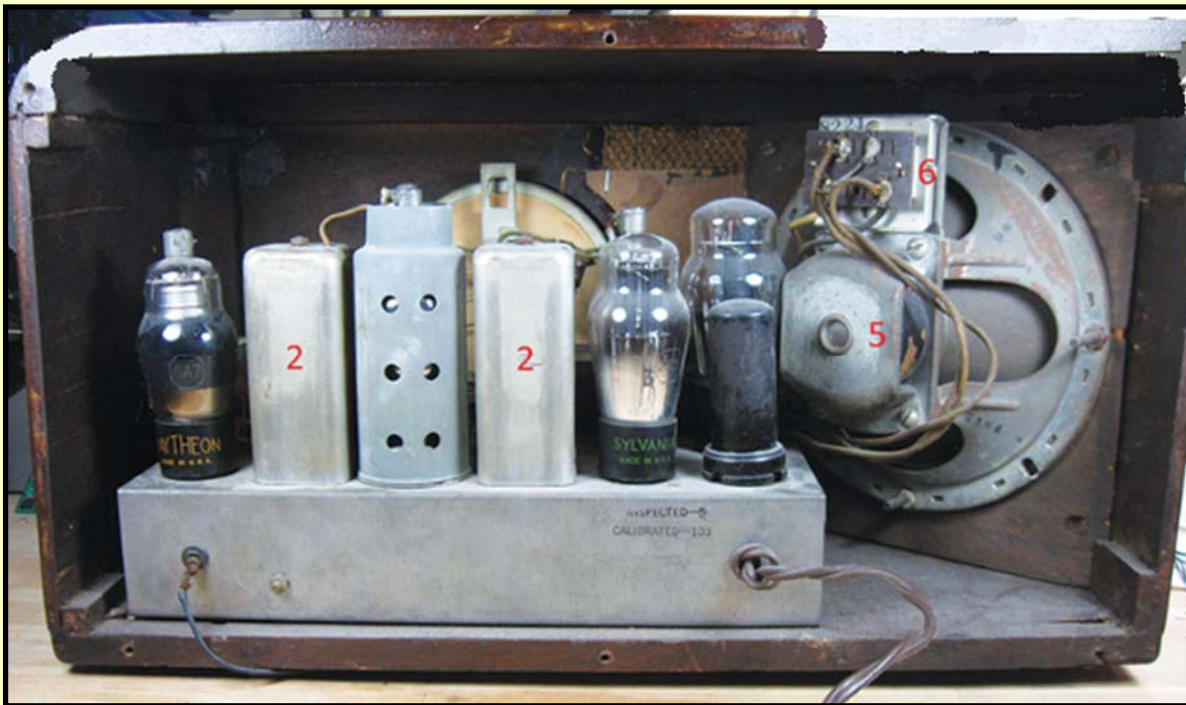
Inside a table model radio showing the vacuum tubes and speaker.
